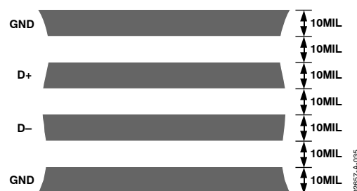
Figure 35. Arrangement of Signal Tracks
