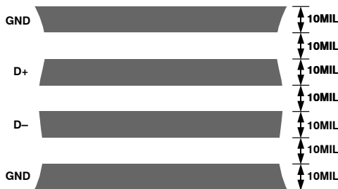
Figure 34. Arrangement of Signal Tracks
