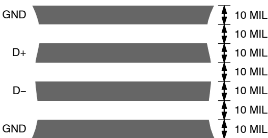
Figure 18. Typical Arrangement of Signal Tracks
