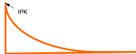
Figure 26. Input Charge Inrush Current
