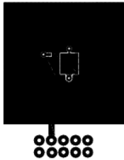
a. 60 °C/W when mounted on a 1 in 2 pad of 2 oz copper
