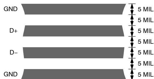
Figure 22. Typical Arrangement of Signal Tracks
