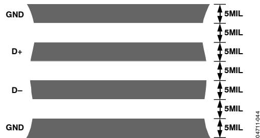
Figure 25. Arrangement of Signal Tracks
