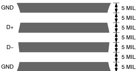
Figure 21. Typical Arrangement of Signal Tracks
