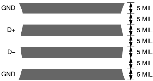
Figure 21. Typical Arrangement of Signal Tracks
