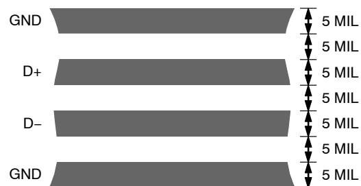
Figure 16. Arrangement of Signal Tracks
