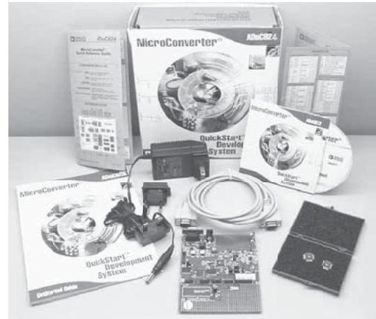
Figure 47. Components of the QuickStart Development System
