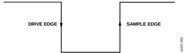
Figure 38. SPI Mode 3 SCLK Edges
