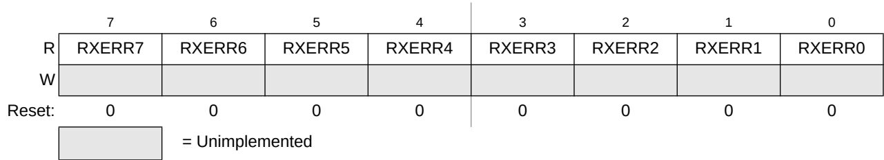
Figure 12-17. MSCAN Receive Error Counter (CANRXERR)
