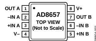
Figure 1. AD8657 Pin Configuration, 8-Lead MSOP
