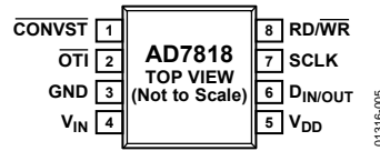
Figure 5. AD7818 Pin Configuration
