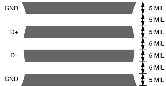
Figure 12. Typical Assignment of Signal Tracks
