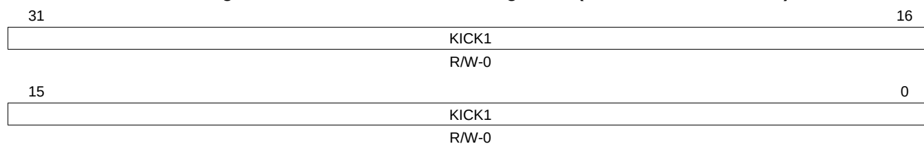
Figure 4-7. KICK_REG1: Kicker Register 1 (Address = FFFFEA3Ch)
