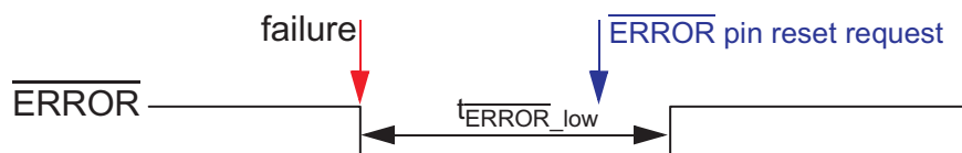
Figure 12-5. \overline{\text{ERROR}} Pin Timing - Example 2
