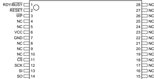
TSOP Top View Type 1
