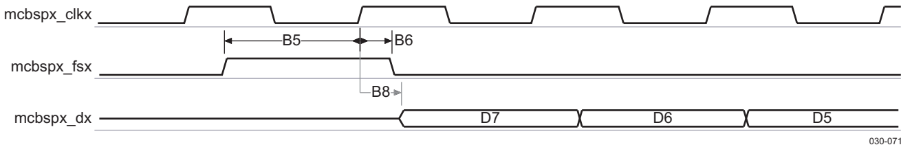
Figure 6-40. McBSP Rising Edge Transmit Timing in Slave Mode
