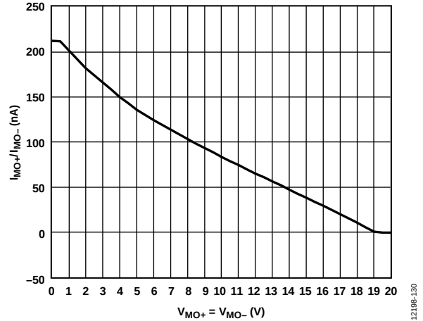
Figure 40. I_{MO+}/I_{MO-} vs. V_{MO+}/V_{MO-} with V_{CC} = 20\text{ V}
