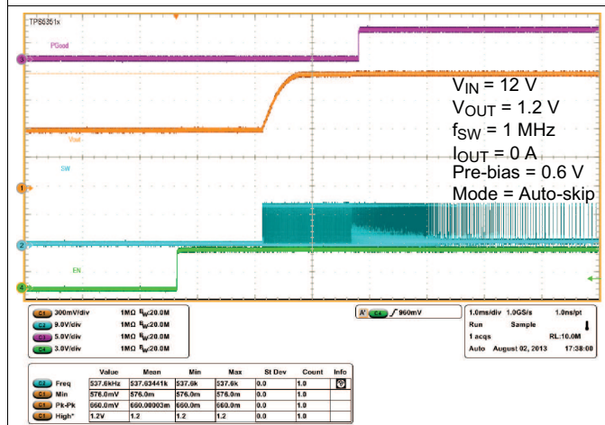
Figure 27. Auto-Skip Mode Shutdown Operation
