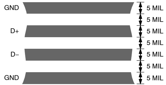
Figure 22. Typical Arrangement of Signal Tracks
