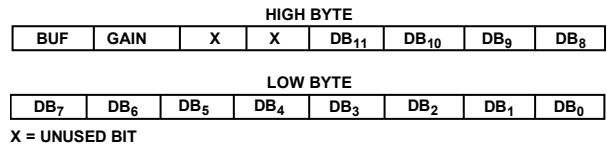
Figure 42. AD5341 with GAIN and BUF Data on 8-Bit Bus
