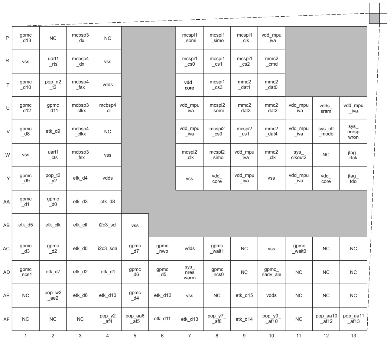
Figure 2-12. CBC Pin Map [Quadrant C - Top View]
