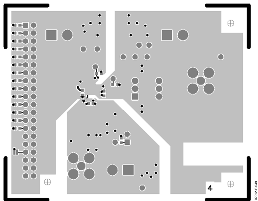
Figure 50. LFCSP Evaluation Board Layout—Secondary Side
