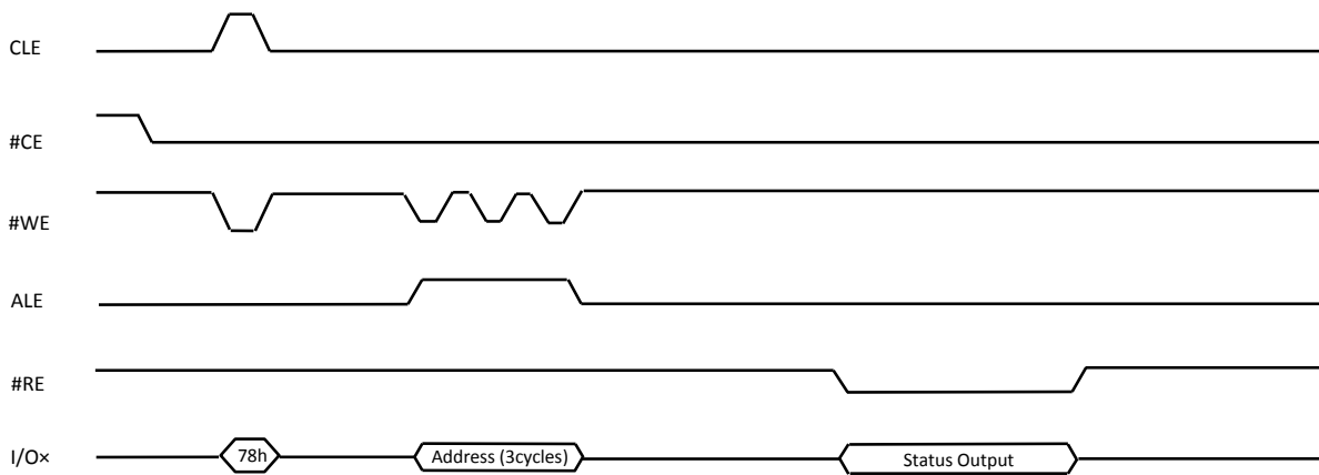
Figure 9-10 Read Status Enhanced (78h) Operation
