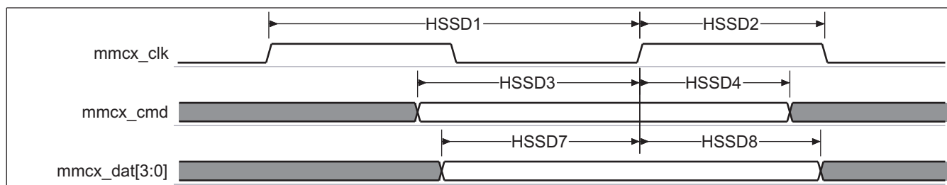
Figure 6-68. MMC/SD/SDIO High-Speed SD Mode Data/Command Receive
