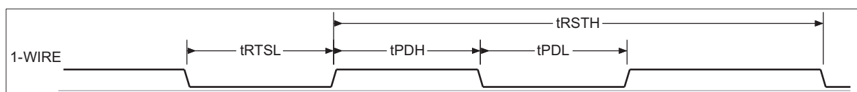
Figure 6-61. 1-Wire Break (Reset) Timing
