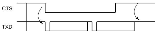
Figure 21-28. Transmitter Behavior when Operating with Hardware Handshaking
