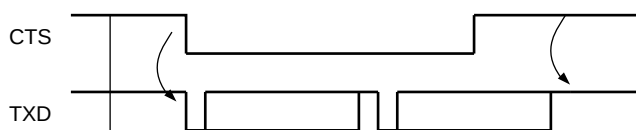
Figure 25-28. Transmitter Behavior when Operating with Hardware Handshaking
