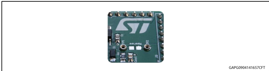
Figure 4: Mounting through-hole sense resistor
