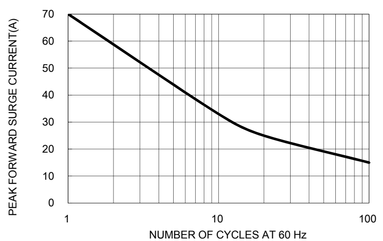
FIG. 2 MAXIMUM FORWARD SURGE CURRENT
