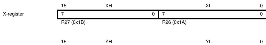
Figure 4-3. The X-, Y-, and Z-registers
