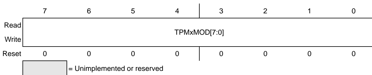
Figure 18-9. Timer/PWM Counter Modulo Register High (TPMxMODH)
