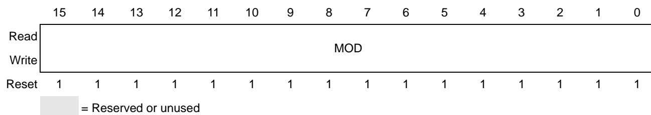
Figure 13-6. PDB Modulus register (MOD)
