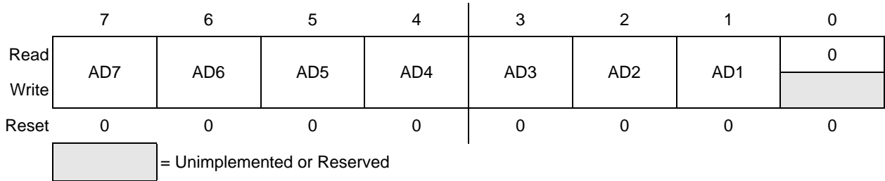
Figure 9-2. I 2 C Address Register 1 (IICA1)
