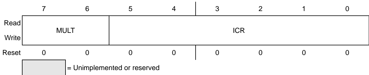
Figure 9-3. I 2 C Frequency Divider register (IICF)
