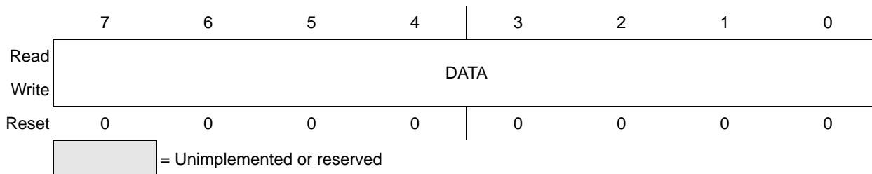
Figure 9-6. I 2 C Data I/O register (IICD)
