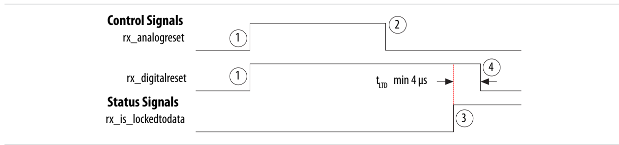
Figure 3-8: Reset Sequence Timing Diagram for Receiver using the User-Coded Reset Controller during Device Operation
