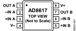
Figure 2. 8-Lead MSOP and 8-Lead SOIC_N
