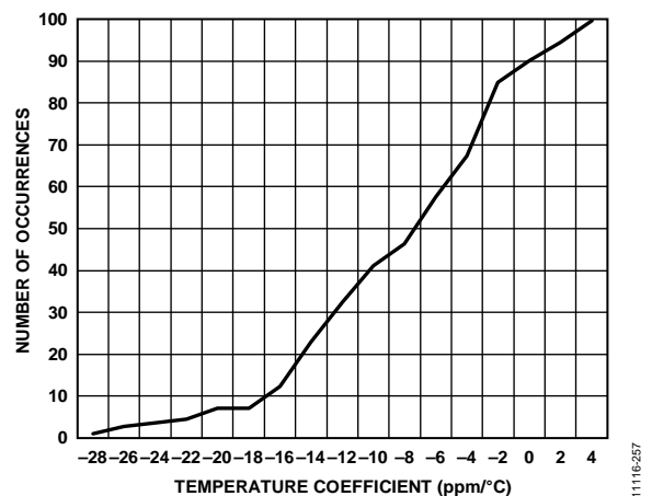
Figure 41. Cumulative Histogram of the ADE7933/ADE7923 Voltage Channel V2 ADC Gain Temperature Coefficient for Temperatures Between +25^{\circ}\text{C} and +85^{\circ}\text{C}
