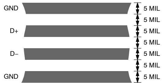
Figure 28. Arrangement of Signal Tracks
