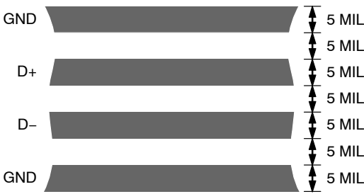
Figure 21. Typical Arrangement of Signal Tracks
