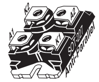
ISOTOP® [J] SOT-227 Antiparallel Configuration (Isolated Base)
