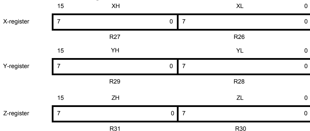
Figure 12-3. The X-, Y-, and Z-registers
