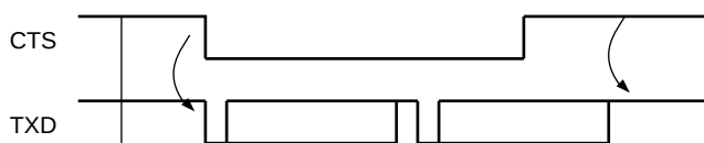
Figure 34-29. Transmitter Behavior when Operating with Hardware Handshaking
