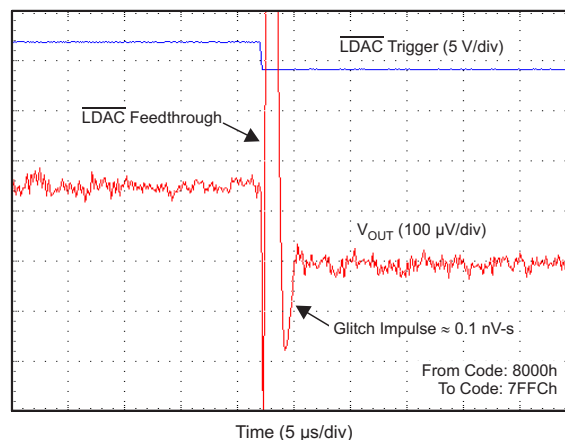
Figure 80. Glitch Impulse, Falling Edge, 1-LSB Step
