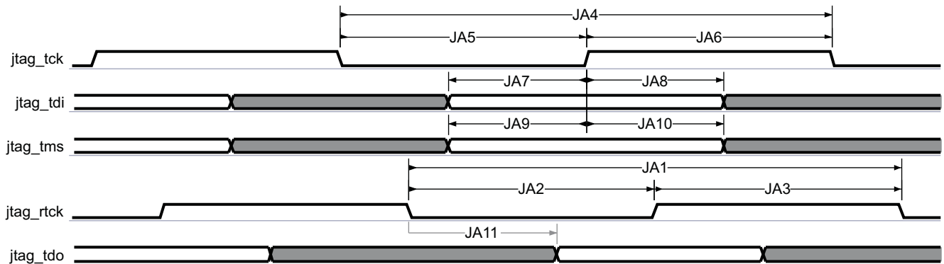
Figure 6-83. JTAG—Adaptative Clock Mode
