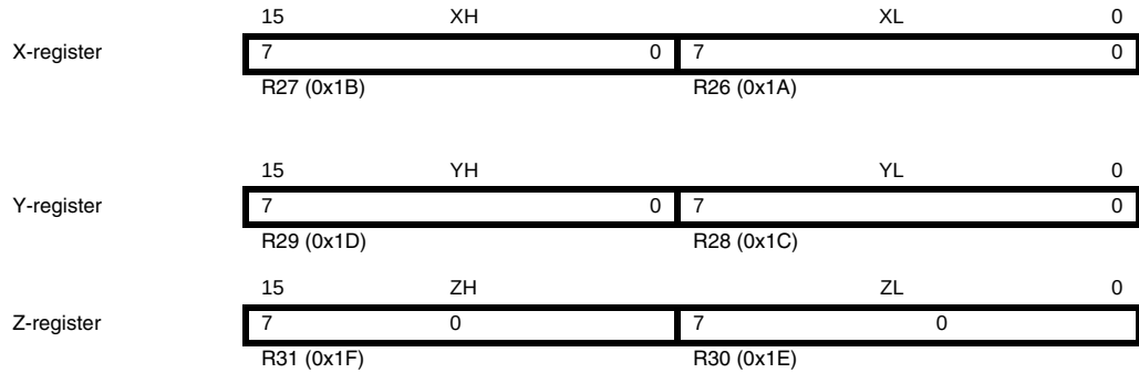
Figure 4-3. The X-, Y-, and Z-registers
