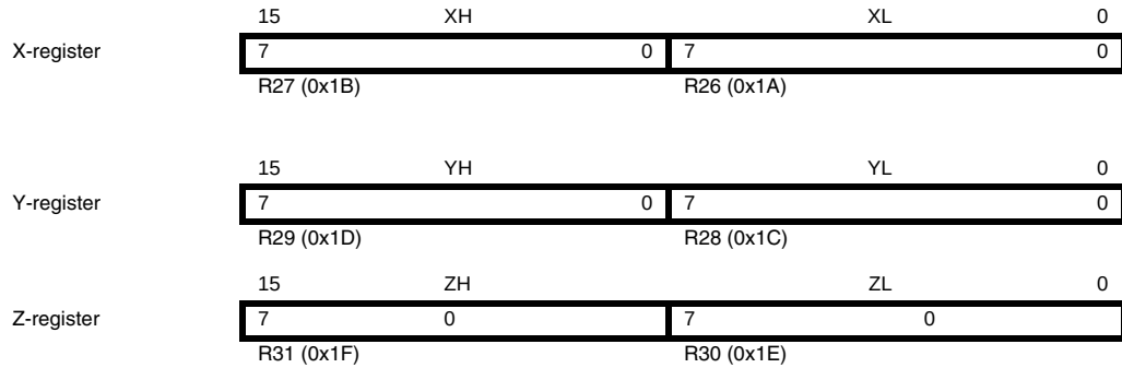
Figure 4-3. The X-, Y-, and Z-registers
