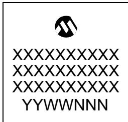
44-Lead QFN (8x8x0.9 mm)
