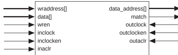
Figure 23. APEX 20KE CAM Block Diagram
