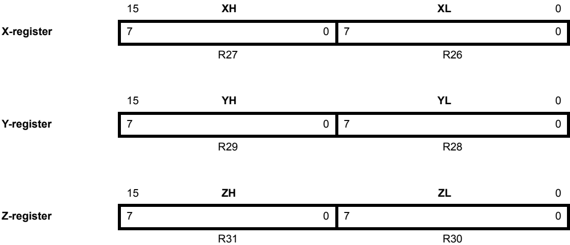
Figure 5-3. The X-, Y-, and Z-registers
