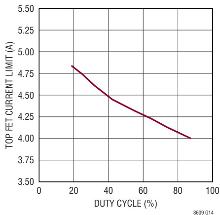
Top FET Current Limit vs Duty Cycle
