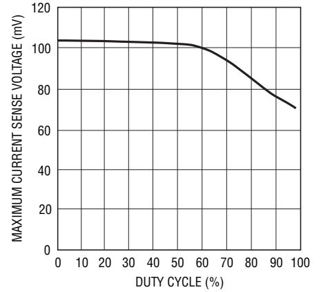
Maximum Current Sense Threshold vs Duty
